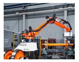
The Krautkrämer WheelStar RPS is a robotic ultrasonic inspection system for dismantled train wheels which uses state-of-the-art matrix phased array technology.
